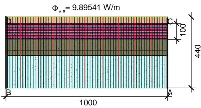
$$U_{\text{eq A-B}} = \frac{\Phi}{\Delta T \cdot b} = \frac{9.895}{30.0 \cdot 1.0} = 0.330 \text{ W/(m}^2 \cdot \text{K)}$$
