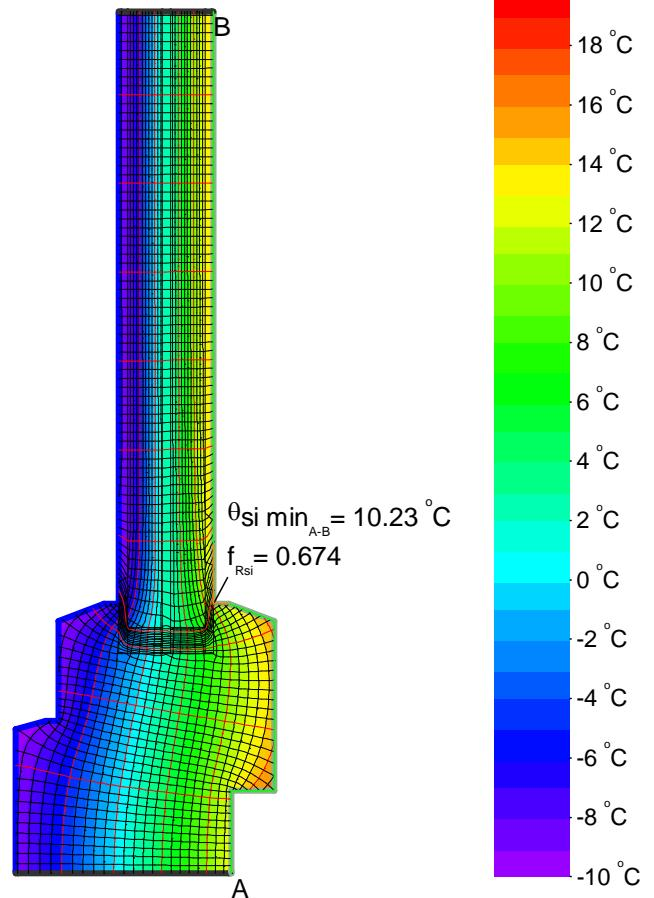
$$\psi_{A-E-C,\cdot} = \frac{\Phi}{\Delta T} - U_1 \cdot b_1 - U_2 \cdot b_2 = \frac{12.01}{30.0} - 0.92 \cdot 0.125 - 0.9 \cdot 0.275 = 0.038 \text{ W}/(\text{m} \cdot \text{K})$$
