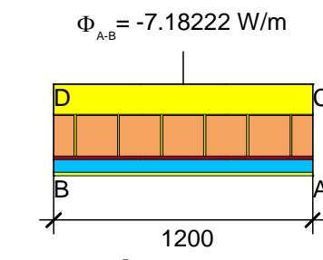
$$U_{eq A-B} = \frac{\Phi}{\Delta T \cdot b} = \frac{7.182}{30.0 \cdot 1.2} = 0.200 \text{ W/(m}^2\cdot\text{K)}$$
