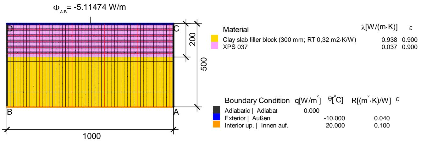
$$U_{\text{eq A-B}} = \frac{\Phi}{\Delta T \cdot b} = \frac{5.115}{30.0 \cdot 1.0} = 0.170 \text{ W}/(\text{m}^2 \cdot \text{K})$$
