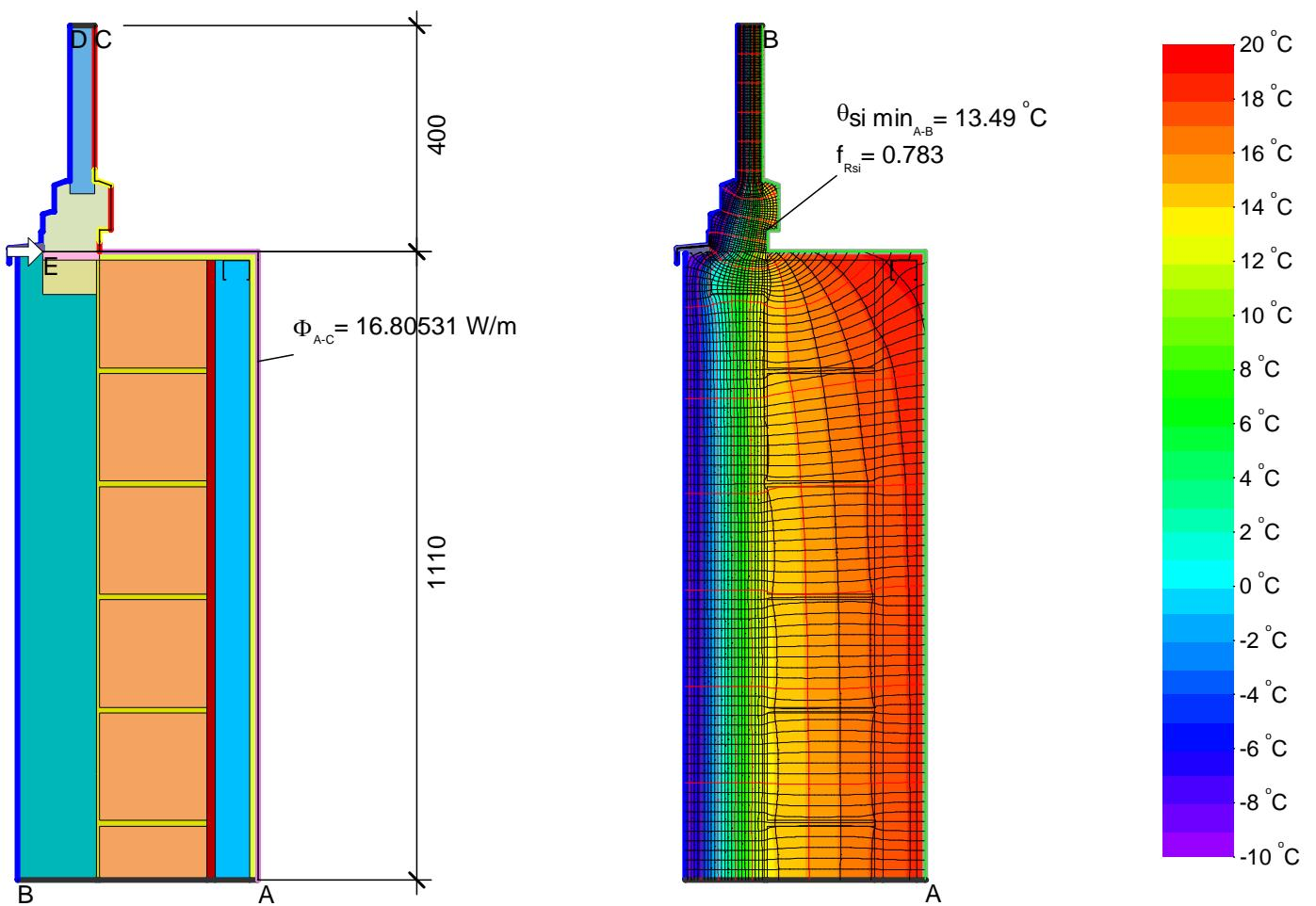
$$\psi_{A-E-C,\cdot} = \frac{\Phi}{\Delta T} - U_1 \cdot b_1 - \frac{\Phi_2}{\Delta T} = \frac{16.805}{30.0} - 0.2 \cdot 1.11 - \frac{9.23}{30.0} = 0.031 \text{ W/(m}\cdot\text{K)}$$
