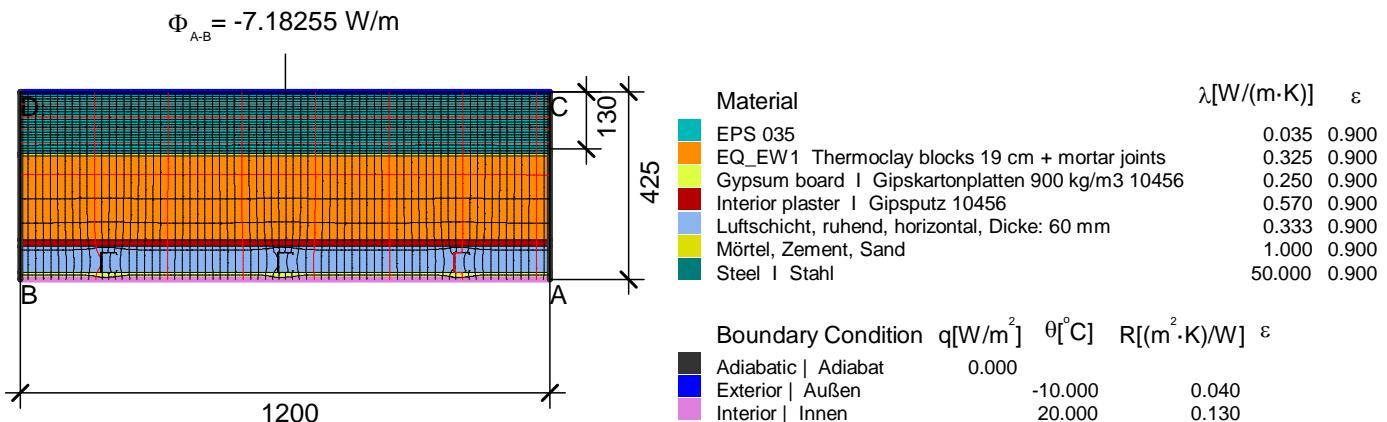
$$U_{eq A-B} = \frac{\Phi}{\Delta T \cdot b} = \frac{7.183}{30.0 \cdot 1.2} = 0.200 \text{ W}/(\text{m}^2 \cdot \text{K})$$
