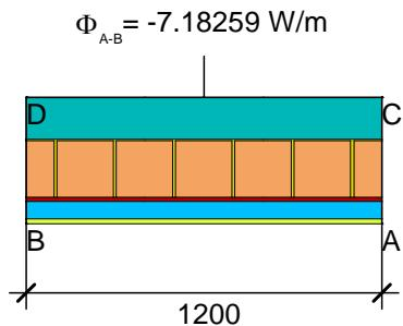
$$U_{eq A-B} = \frac{\Phi}{\Delta T \cdot b} = \frac{7.183}{30.0 \cdot 1.2} = 0.200 \text{ W/(m}^2\cdot\text{K)}$$
