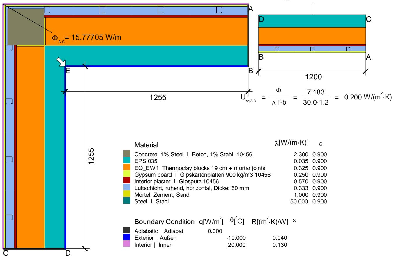
$$\psi_{A-E-C, \cdot} = \frac{\Phi}{\Delta T} - U_1 \cdot b_1 - U_2 \cdot b_2 = \frac{15.777}{30.0} - 0.2 \cdot 1.255 - 0.2 \cdot 1.255 = 0.025 \text{ W/(m} \cdot \text{K)}$$
