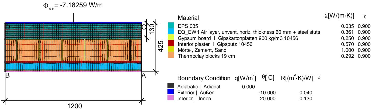
$$U_{eq A-B} = \frac{\Phi}{\Delta T \cdot b} = \frac{7.183}{30.0 \cdot 1.2} = 0.200 \text{ W}/(\text{m}^2 \cdot \text{K})$$
