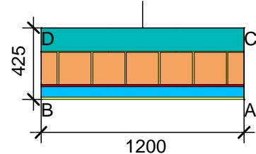
$$U_{eq A-B} = \frac{\Phi}{\Delta T \cdot b} = \frac{7.183}{30.0 \cdot 1.2} = 0.200 \text{ W/(m}^2 \cdot \text{K)}$$
