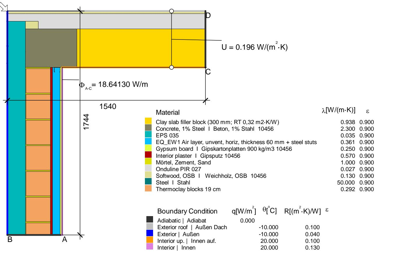
$$\psi_{A-E-C,-} = \frac{\Phi}{\Delta T} - U_1 \cdot b_1 - U_2 \cdot b_2 = \frac{18.641}{30.0} - 0.2 \cdot 1.744 - 0.196 \cdot 1.54 = -0.028 \text{ W}/(\text{m} \cdot \text{K})$$
