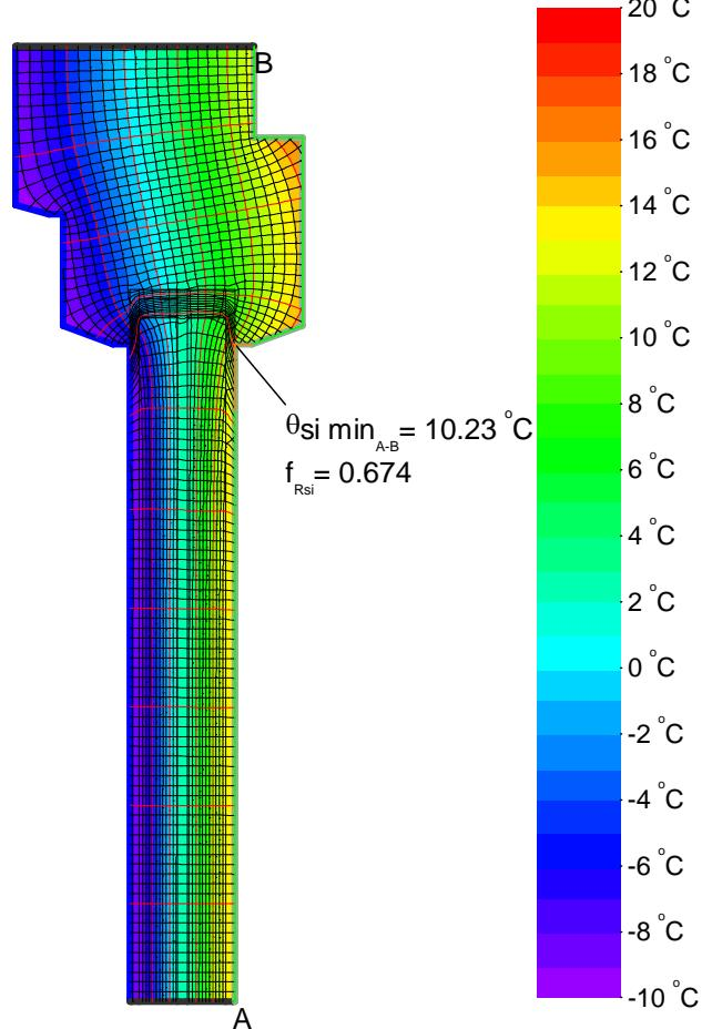
$$\psi_{A-E-C,\cdot} = \frac{\Phi}{\Delta T} - U_1 \cdot b_1 - U_2 \cdot b_2 = \frac{12.01}{30.0} - 0.9 \cdot 0.275 - 0.92 \cdot 0.125 = 0.038 \text{ W/(m}\cdot\text{K)}$$
