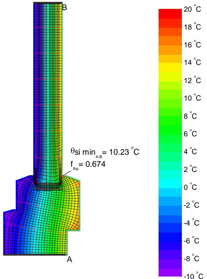
$$\psi_{A-E-C, \dots} = \frac{\Phi}{\Delta T} - U_1 \cdot b_1 - U_2 \cdot b_2 = \frac{12.01}{30.0} - 0.92 \cdot 0.125 - 0.9 \cdot 0.275 = 0.038 \text{ W}/(\text{m} \cdot \text{K})$$
